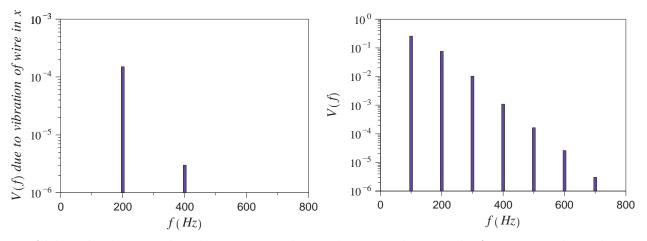
Although the wire has been assumed to vibrate with a single frequency, the voltage waveform V(t) is nearly triangular in shape. Recall that a plucked string has a triangular waveform [13], so the "distortion" of an electric guitar pickup tends to "sharpen" the plucked sound of the instrument, which has proven to be a very popular effect.
