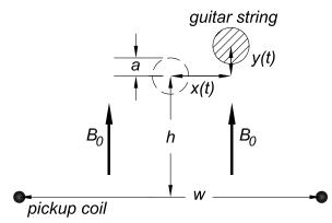
Deduce the magnetic field when the string is displaced by (x, y) from its rest position, and from this deduce the voltage V(t) induced in the pickup coil by the vibrating string.
