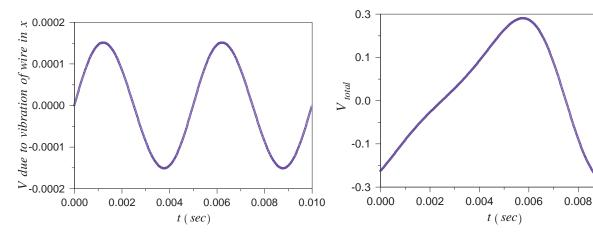
A Fourier analysis [12] of these voltage waveforms is shown in the figures below. The left figure is the voltage due to the x vibration of the string, and has significant frequency components only at the second and fourth harmonics. The right figure is the total induced voltage (almost entirely due to the y vibration of the string), which contains frequency components at all harmonics of the fundamental, with exponentially decreasing strength as a function of the harmonic number.
